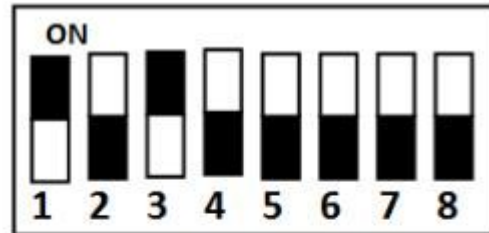
Address 5 - Door 3 Entrance Card Reader
